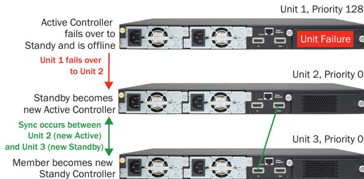
**Figure 2.** New stack configuration after hitless failover.
