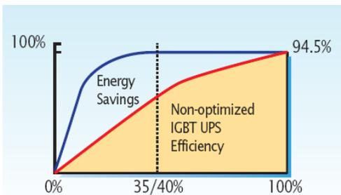
MGE™ EPST™ 8000 features a high efficiency rate that remains stable even at lower loads where most UPSs operate. The energy cost savings usually exceeds the value of the UPS in as little as three to five years. The efficiency shown above is the core efficiency without the input isolation transformer for comparison purposes.
