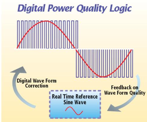
Another benefit of the high-resolution control topology is that harmonic distortion reflected from the loads is practically eliminated. The error correction pulses counteract the reflected waveform distortion reducing THD to under 4%.
