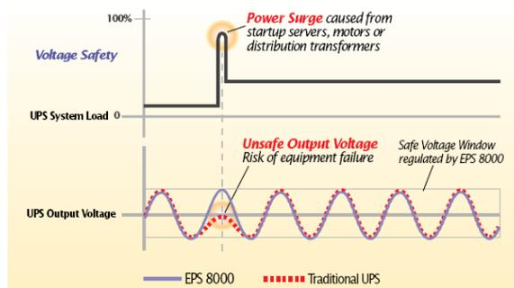
This regulated dynamic response is essential as extreme step loads are common when starting distribution transformers or large banks of servers. Medical imaging systems and broadcast transmitters also exhibit very high step loads making the MGE™ EPS™ 8000 ideal for such applications.
