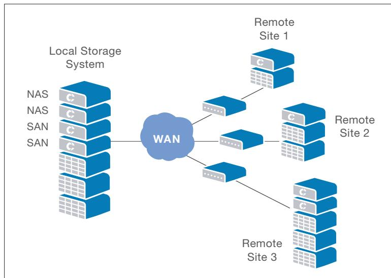
**New Levels of Business Continuity:** Multi-site replication enables robust data protection without the need for matching configurations at each site.
