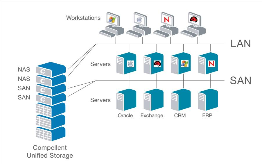
**Unified Storage:** Storage Center with NAS combines block and file-level storage into a single shared system to lower storage costs.
