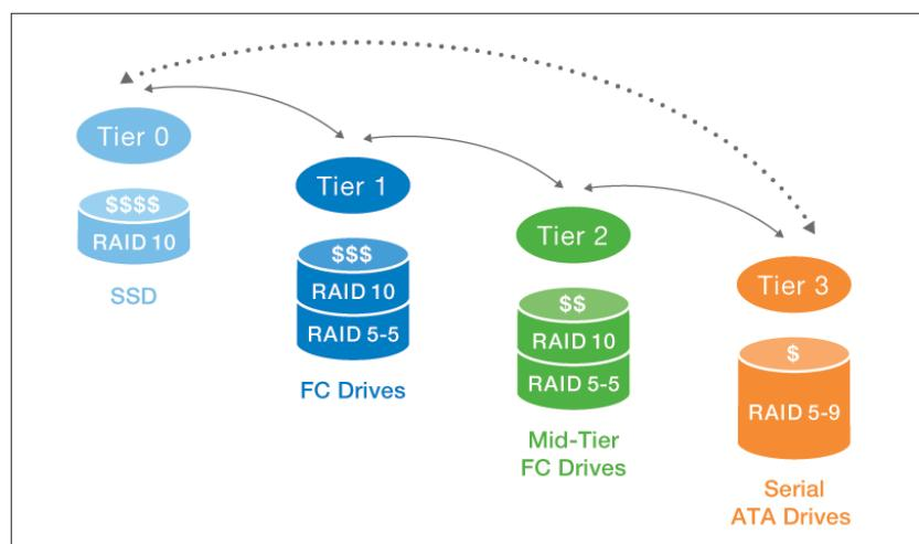
*Optimize File Storage: Data Progression automatically retains frequently accessed data on high performance storage and stores infrequently accessed data on lower cost storage.*
