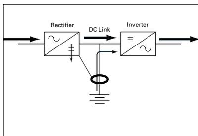
During the battery test, the rectifier regulates DC link voltage to obtain consistent battery power discharge month to month.
