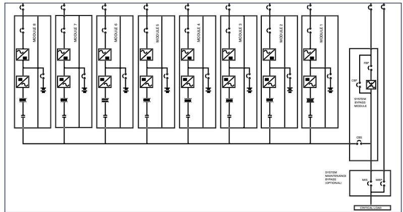
**Powerware Hot Sync – Capacity /Redundant**
