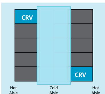
For data centers where heat density needs to be increased without installing a raised floor or a higher roof, the Liebert CRV and Emerson Network Power SmartAisle cold aisle containment is the ideal solution.
