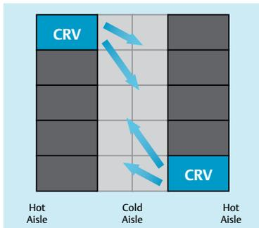
Liebert CRV systems operating in hot aisle/cold aisle configuration.
