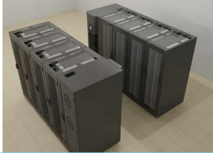
**How It Works.** Used in a hot aisle/cold aisle layout, the Liebert CRV pulls air from the hot aisle, filters and conditions it, and then delivers cool air to the front of equipment racks. Adjustable supply air baffles direct cool air to the left, right, or both sides as needed.
