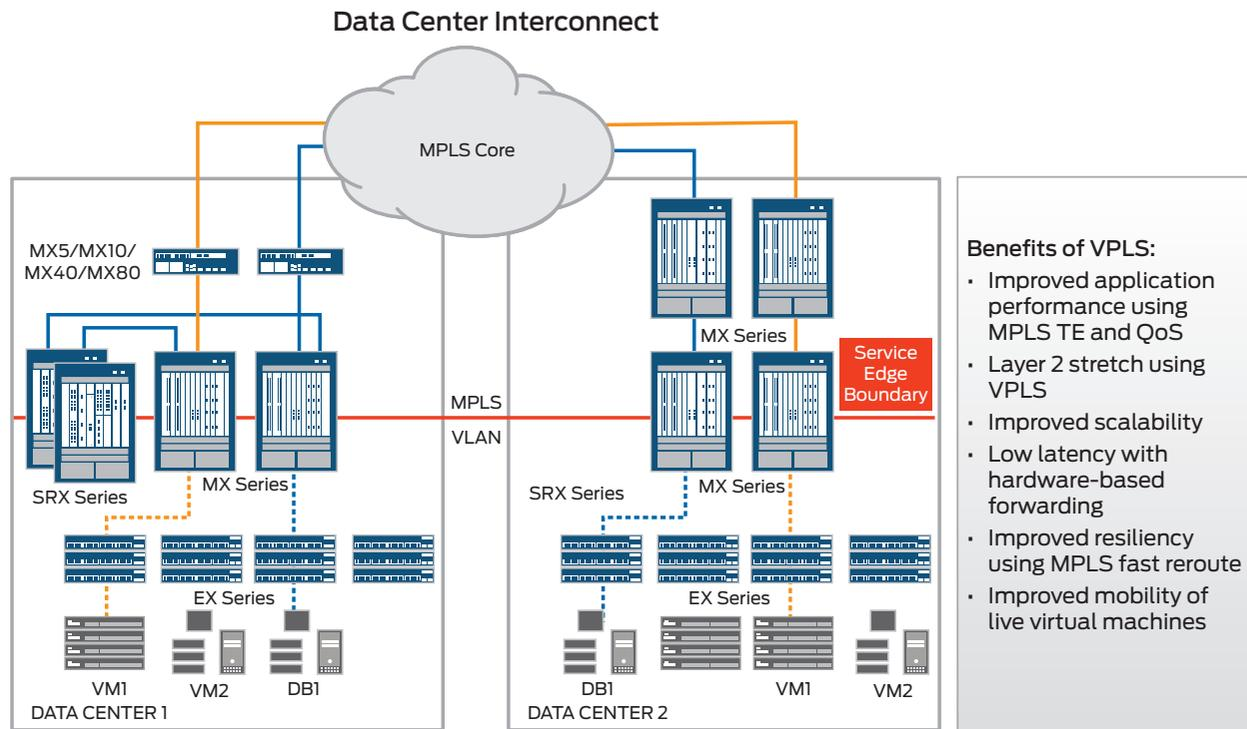
Figure 4: Example of sharing across two data centers using VPLS over MPLS and showing the positioning of compact midrange routers and high-end MX Series devices
