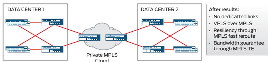
Figure 2 After: Example of the customer with a virtualized network that eliminates dedicated links and delivers 100% improvement in utilization
