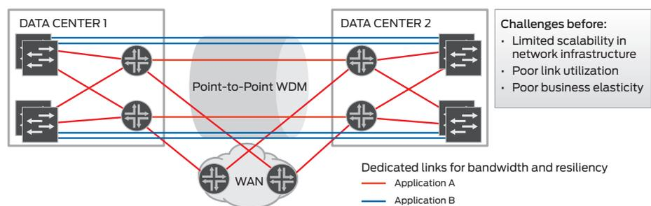
Figure 1: Before: Example of a real customer with 20 x 10GbE dedicated links by application, resulting in 1% utilization
