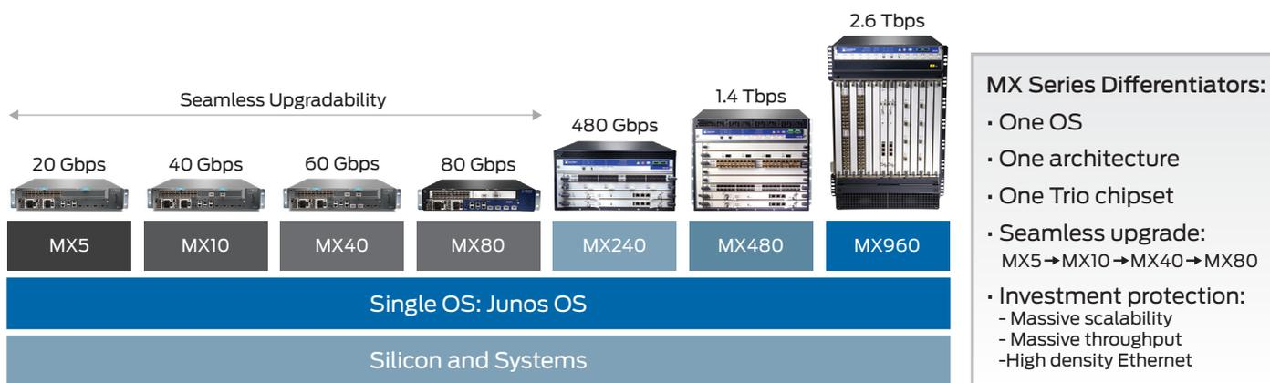
Figure 3: MX Series enterprise WAN routing portfolio simplifies the WAN using one Junos OS, the same Trio silicon, and a consistent architecture
