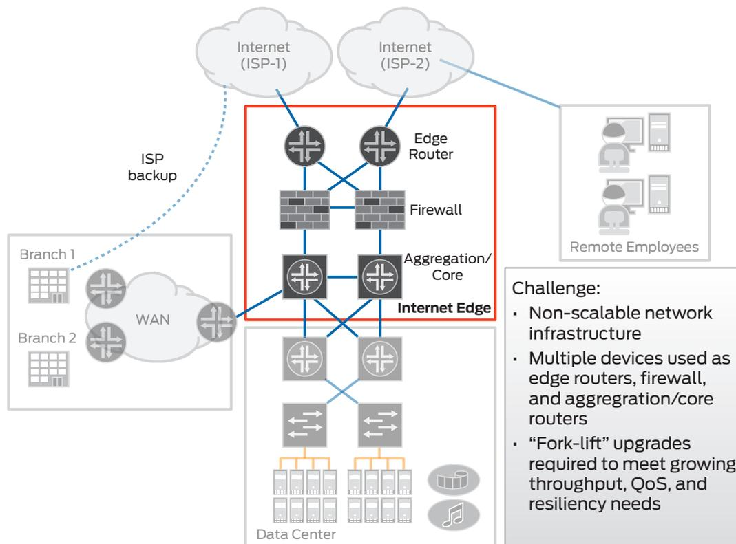
Figure 1: Before—Internet Edge with multiple devices connecting branch offices to the Internet, and remote workers connecting via the Internet
