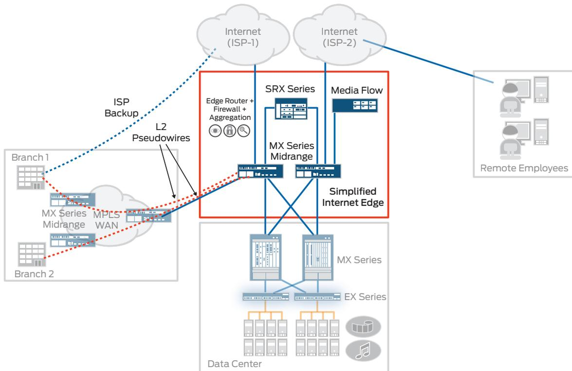
Figure 2: After—Simplified Internet edge consolidates edge, aggregation, and core devices and enables massive upgradeability
