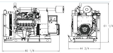
Drawing above for illustration purposes only, based on standard open power 480 volt engine-generator set. Lengths may vary with other voltages. Do not use for installation design. See website for unit specific template drawings.
