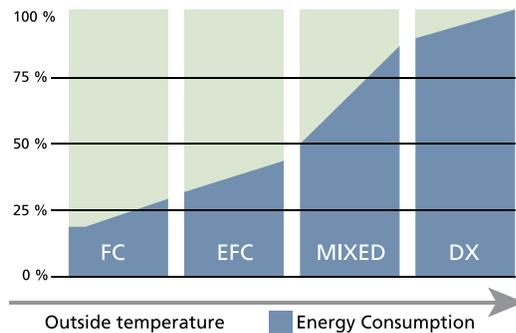
In cool weather, DFC makes use of economical indirect free cooling, which extracts all its cooling power from the outside air. Energy-intensive compressor cooling (DX) is only switched on when absolutely necessary.
